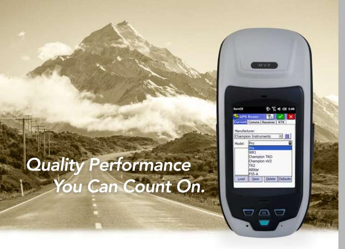
The MVP features the Trimble BD920 receiver module supporting multiple constellations. This delivers the quickest and most reliable RTK initializations for 1-2 centimeter positioning. For applications that do not require centimeter accuracy, the BD920 contains an advanced kalman filter PVT engine that delivers high accuracy GNSS, DGNSS positions in the most challenging environments such as urban canyons.
